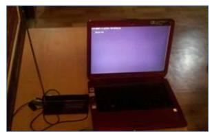
Above is the image of a portable FM receiver hooked up to the Mic input of a laptop. Another laptop's audio line-out was connected to an FM transmitter.
