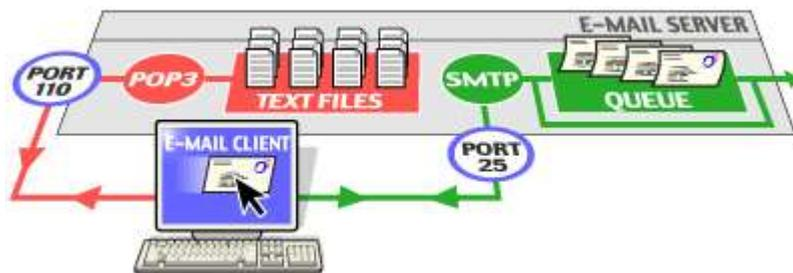
Figure **ERROR! NO SEQUENCE SPECIFIED.** – The above picture shows the working of a real world email system. it represents the workflow of an email.
