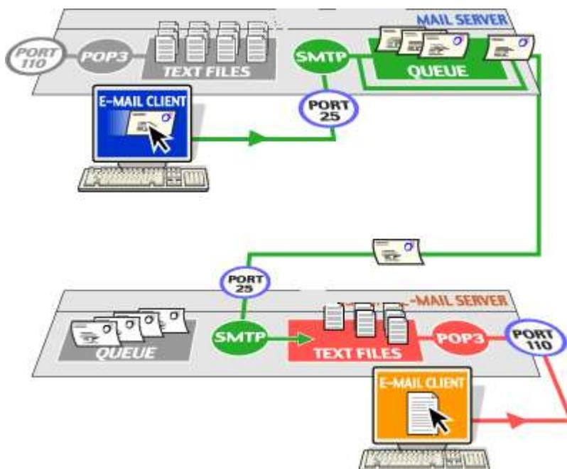
Figure **ERROR! NO SEQUENCE SPECIFIED.** – The above picture shows the working of an smtp server and the workflow when we send an email
