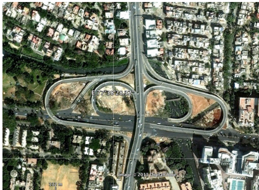
Figure 31: Large Road Projects disrupt the Morphology of Cities; A Clover Leaf in Bangalore
