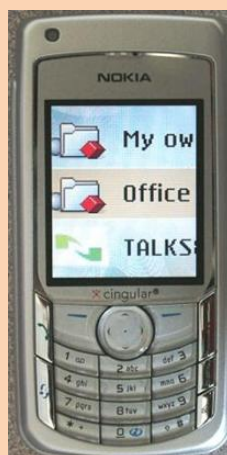
Figure 1.6: Magnifying screens allow users with low vision to enlarge fonts and images.
