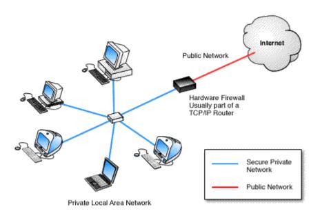
Figure 2: Computer with Firewall Software.
