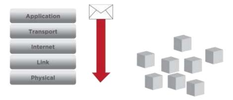
Figure **ERROR! NO SEQUENCE SPECIFIED.** – The picture above shows how messages are broken down into chunks of data and their progression through the layers.
