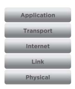
Figure **ERROR! NO SEQUENCE SPECIFIED.** – The picture above shows different layers in a stack of protocols.
